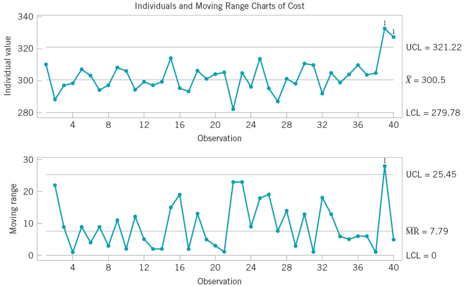
FIGURE 6.20 Continuation of the control chart for individuals and the moving range using the additional data in Table 6.7.
