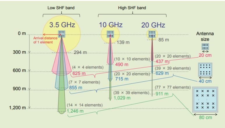
Figure 3 Beamforming effect
