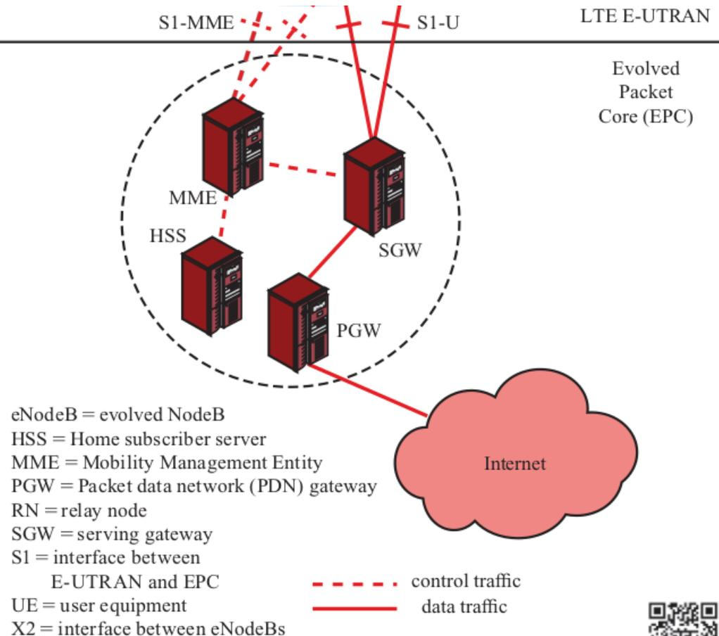
Figure 14.2 Overview of the EPC/LTE Architecture
