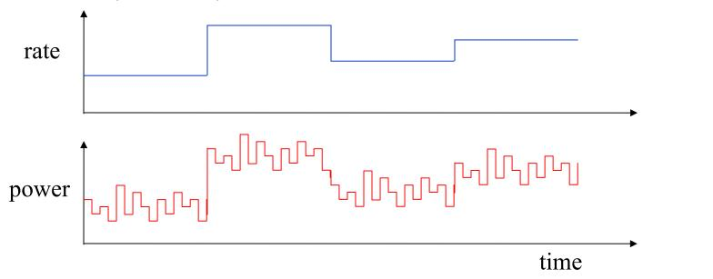
• Outer loop power control (BS-RNC) adjusts target  $E_b/N_0$  to achieve specific frame or block error rate
