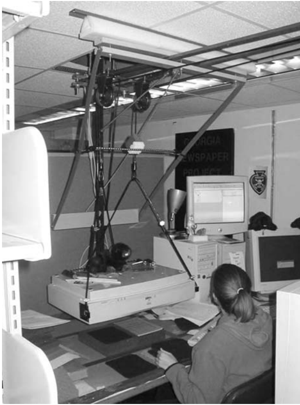
Figure 3.2 Suspending a flatbed scanner to get “look-down” operation.
