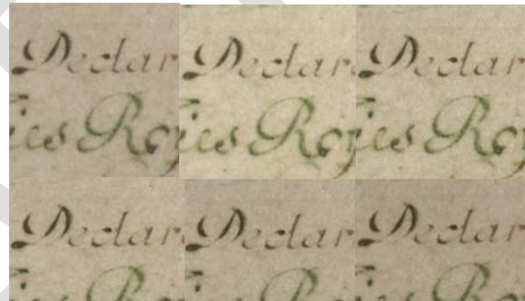
Above: Image blown up 9x increasing resolution from 200-ppi on the left to 700-ppi on the right
