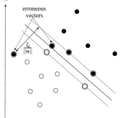
By allowing an error (slack) per training example, we may obtain a larger margin, and we may also find a separating hyperplane even when the training data are not linearly separable (e.g., when using a linear SVM).
