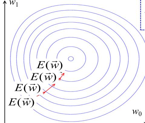
At each iteration, modify  $\vec{w}$  by taking **a step** to the direction  $-\nabla E(\vec{w})$ :
