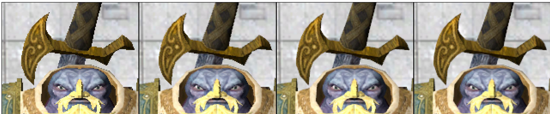
1X (no MSAA), 2X, 4X and 8X coverage samples on an NVIDIA 780Ti graphics card
