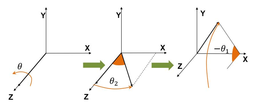
Do the rotation around z instead ... and revert to the  $\vec{v}$  axis
