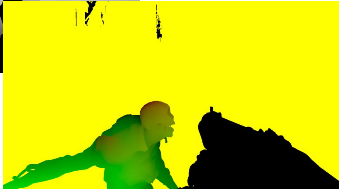
Velocity buffer 2 float channels: dx, dy
