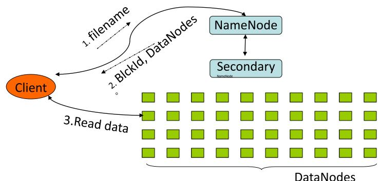
NameNode : Maps a file to a file-id and list of DataNodes DataNode : Maps a block-id to a physical location on disk
