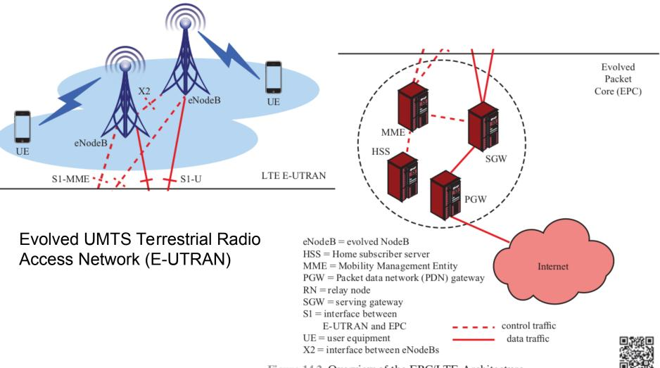
Figure 14.2 Overview of the EPC/LTE Architecture
