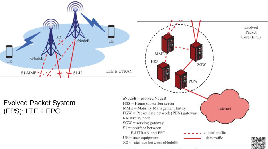
Figure 14.2 Overview of the EPC/LTE Architecture
