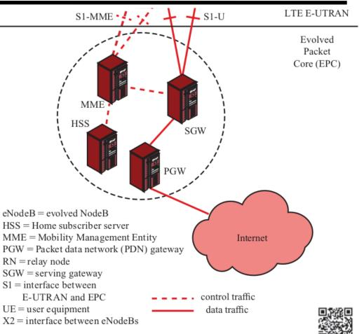
Figure 14.2 Overview of the EPC/LTE Architecture
