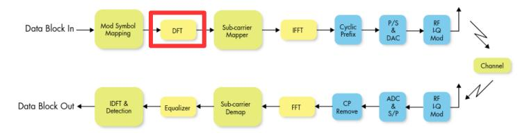
Figure 4. SC-FDMA Transmitter and Receiver
