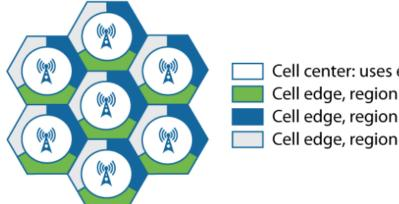
Cell center: uses entire spectrum channel
