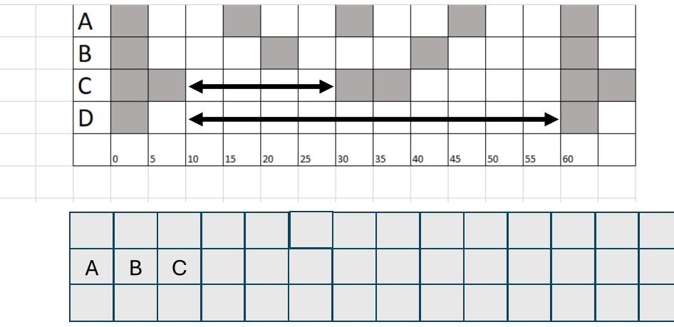
At 10 ms, process C has the shortest deadline and is assigned the highest priority, so it will begin execution during this interval.
