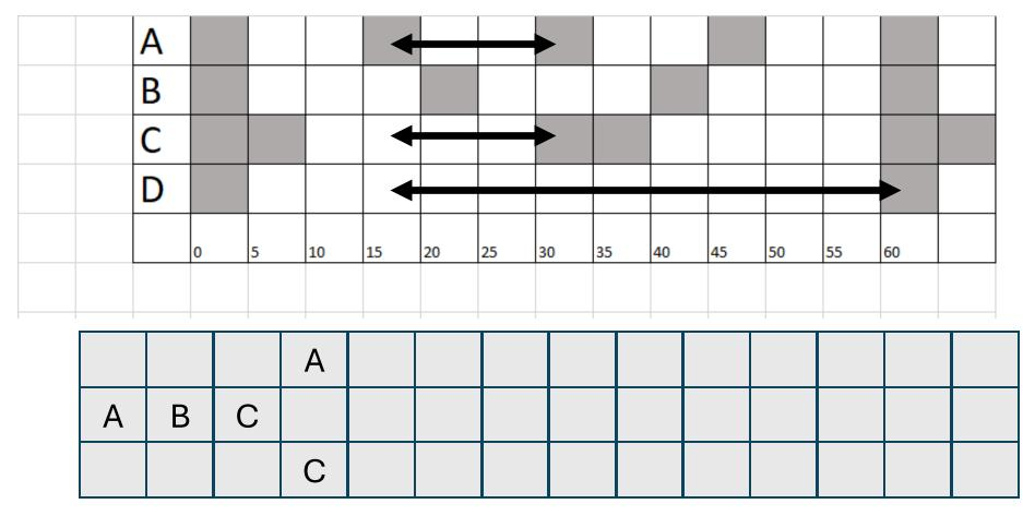
At 15 ms, we have three processes to consider for execution. We can see that processes A and the remaining portion of process C have the same deadline, which is earlier than the deadline of process D. Therefore, both processes A and C are assigned the highest (equal) priority.
