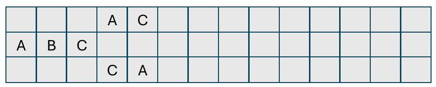
At 20 ms, process B reappears. Since process A or the remainder of process C (whichever has not been selected previously to execute), has the earliest deadline, it is assigned the highest priority and will execute during this interval.
