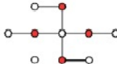
A vertex cover of size 4 optimal solution!!
