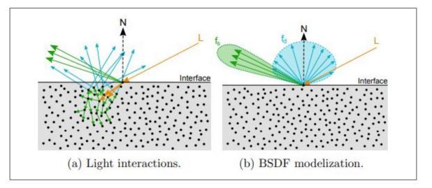
$$L(p,\,\omega_o)\,=\,L_e\,+\,\int_H f(p,\,\omega_o,\,\omega_i)\,L(p,\,\omega_i)\,\cos heta\,d_{\omega_i}$$
