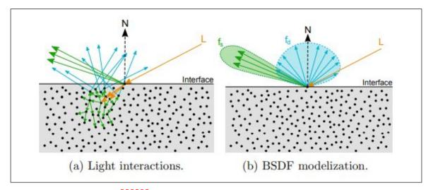
$$L(p,\,\omega_o)\,=\,L_e\,+\,\int_H f(p,\,\omega_o,\,\omega_i)\,L(p,\,\omega_i)\,\cos heta\,d_{\omega_i}$$
