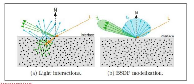
$$L(p,\,\omega_o) \,=\, L_e \,+\, \int_H f(p,\,\omega_o,\,\omega_i) L(p,\,\omega_i) \,\cos heta \, d_{\omega_i}$$
