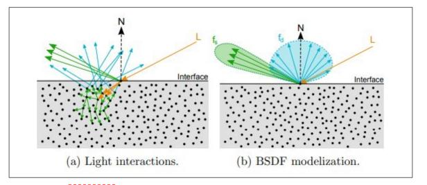
$$L(p,\,\omega_o) \,=\, L_e \,+\, \int_H f(p,\,\omega_o,\,\omega_i) iggl[ L(p,\,\omega_i) iggl] \cos heta \, d_{\omega_i}$$
