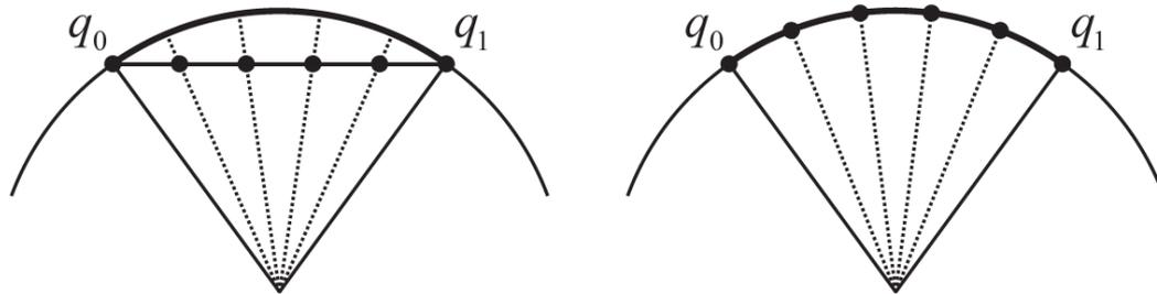
$$q_s(t) = q_0 \frac{\sin(1-t)\omega}{\sin \omega} + q_1 \frac{\sin t\omega}{\sin \omega}, \quad t \in [0,1]$$
