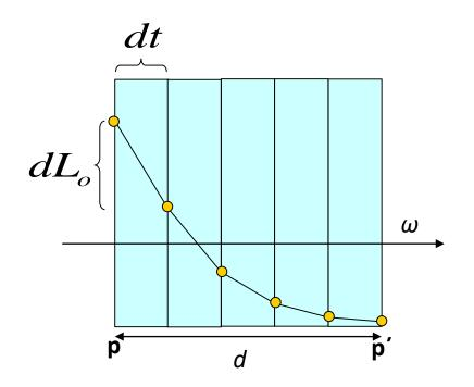
Transmittance: Fraction of light transmitted from **p** to **p**'
