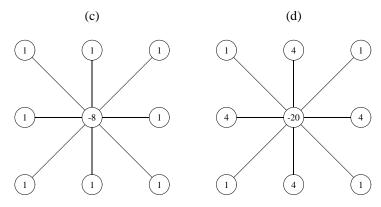
**Figure 2.4** *Two nine-point centered difference stencils for the Laplacean operator.*
