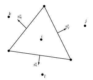
**Figure 2.12** Finite volume cell associated with node *i* and three neighboring cells.
