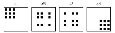
**Figure 2.9** The element matrices  $A^{[e]}$ , e = 1, ..., 4 for the finite element mesh shown in Figure 2.8.
