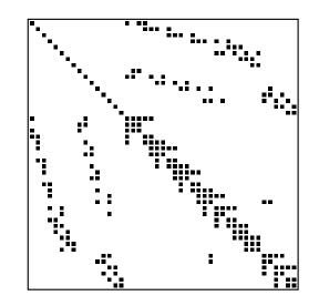
**Figure 3.2** Sparse matrix associated with the finite element grid of Figure 3.1.
