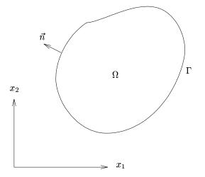
**Figure 2.1** Domain  $\Omega$  for Poisson's equation.
