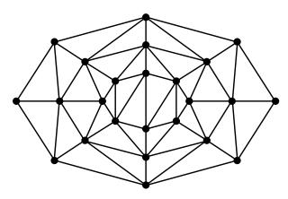
Figure 2.7 Finite element triangulation of a domain.
