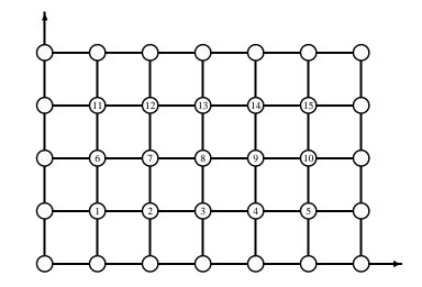
**Figure 2.5** *Natural ordering of the unknowns for a*  $7 \times 5$  *two- dimensional grid.*
