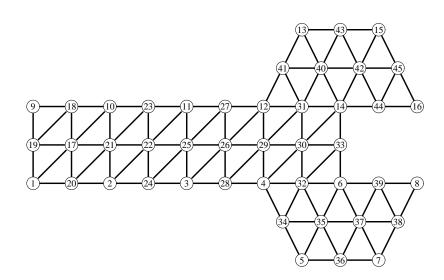
Figure 3.1 A finite element grid model.
