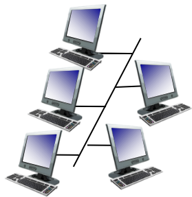
shared wire (e.g., cabled Ethernet)
